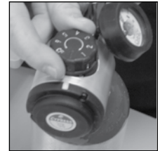
FIGURE F View of the CYPRESS selector switch
